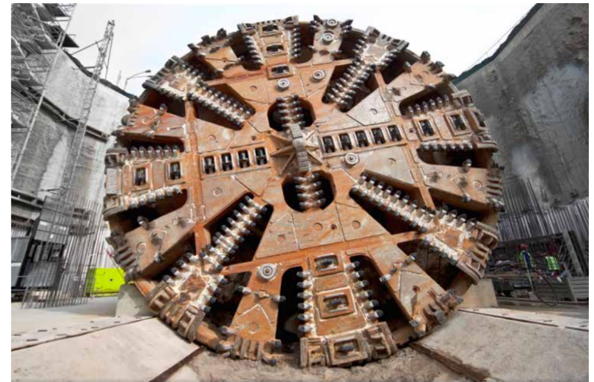
Figure 101 - Tunnel boring machine (TBM) – cutter head
